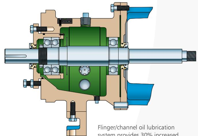
Flinger/channel oil lubrication system provides 30% increased L'10 life; 15°F (8°C) reduced oil temperature.
